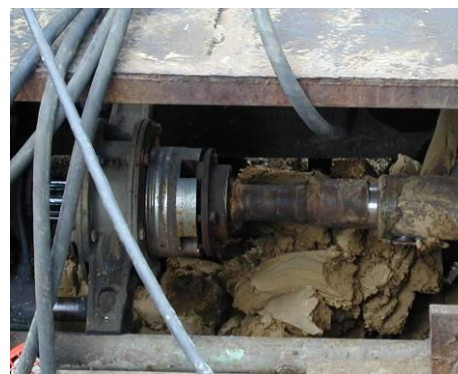
Fig. 4. Typical bearing units of auger equipment: (a) support-centering bearing unit; (b) traverse of the drill slip lock
