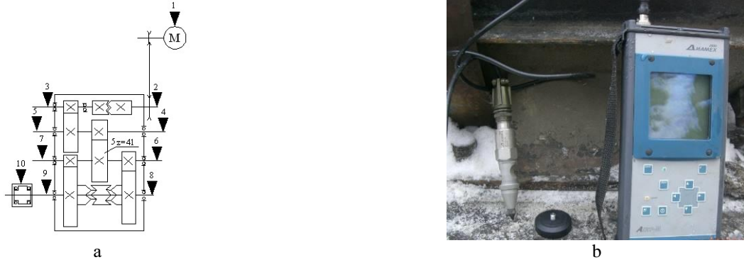
Fig. 5. Scheme of vibration measurement: (a) points on the gear rotator 2-9 – gear bearings, 10 - the bearing assembly tool joint; (b) vibration analyzer «Agat-M»
