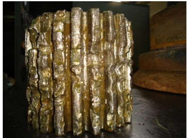
Fig. 5. Defects of the Gear in Harmonic Drive of the Cutting Unit of the Header SM-130
