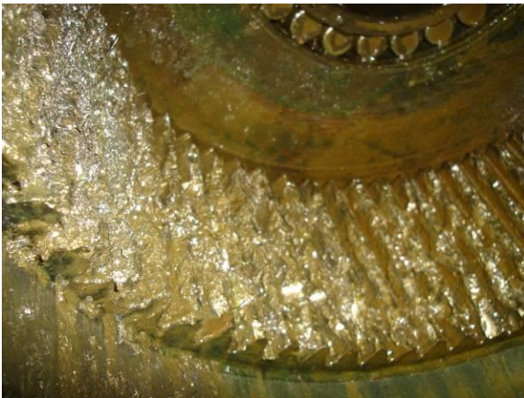
Fig. 5. Defects of the Gear in Harmonic Drive of the Cutting Unit of the Header SM-130
