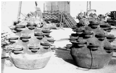
Fig. 1. Cutting drums equipped with disc cutters.
