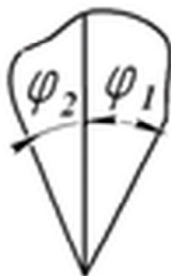
Fig. 2. Biconical cutting disc with asymmetric angles.
