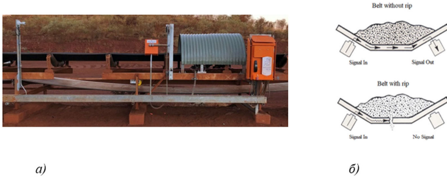
Fig. 4. Probe BG10k, Beltscan; a) installation on conveyor, b) operating principle.
